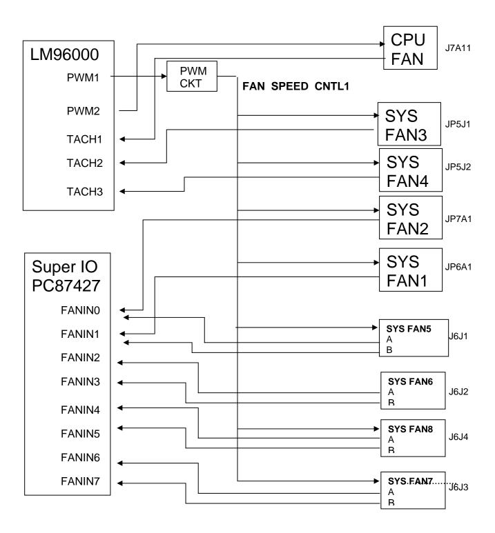
Figure 10. Fan Speed Control Block Diagram
